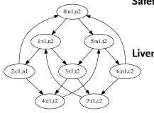
Safety "Only one process is in its critical section at any time."  $\nu Z.\neg(c_1 \wedge c_2) \wedge [a]Z$
